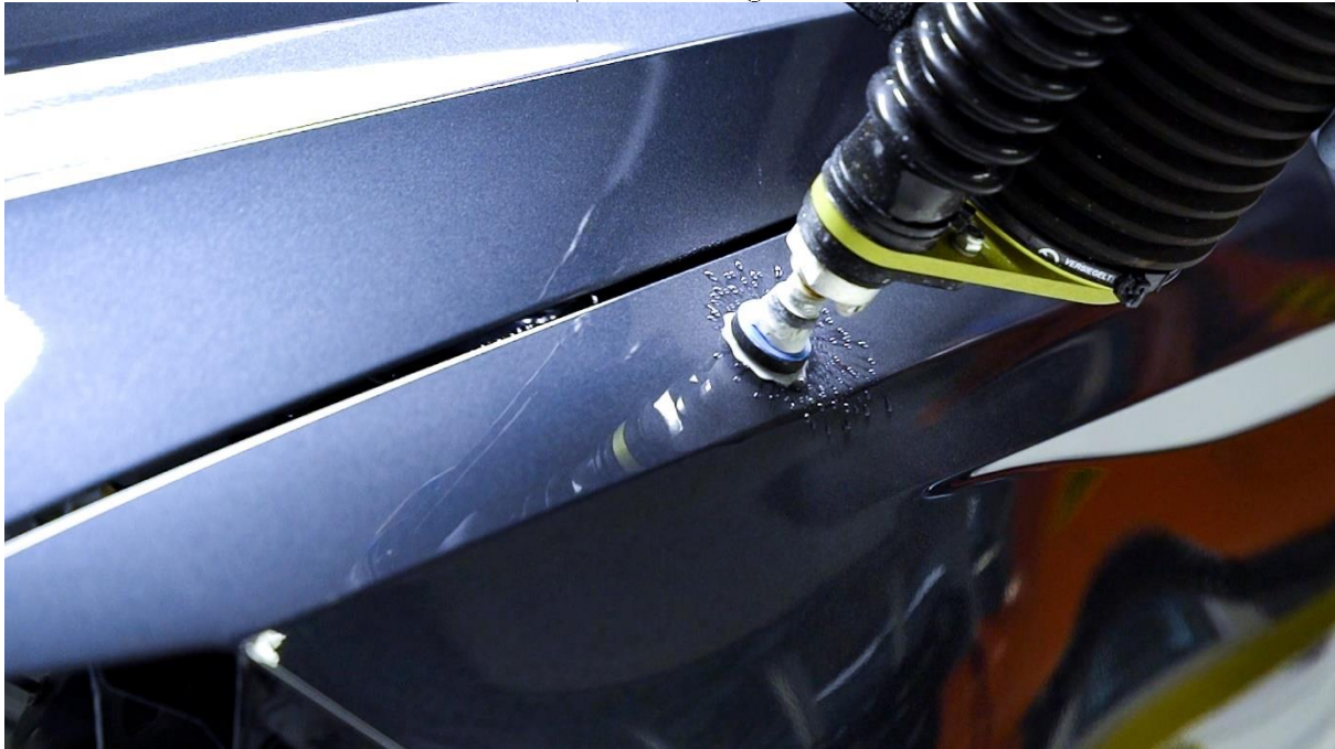
FerRobotics AOK XS (Active Orbital Kit XS) – Ideal for contact sensitive surface finishing.
